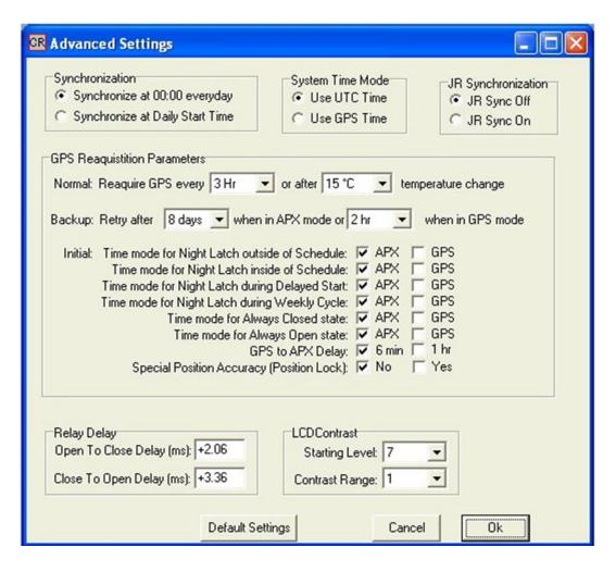
Note: It is highly recommended that you at least begin with the default settings provided by MCM, since the default settings represent the optimum settings regarding balancing battery power consumption and clock accuracy. The default settings are indicated on the above window. If you make changes and decide to return to the default settings, you can click on the "Default Settings" button on the above window.
